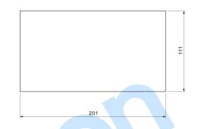
Fig.26 – HPM6D Display Module Installation Dimensions (Unit: mm)
