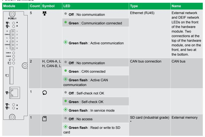
NOTE \* To meet the temperature and EMC specifications, you must use an industrial grade SD card.
