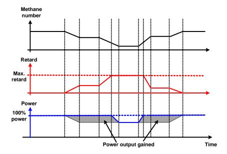
So, from the start of the retard until maximum retard is reached, there will be no change in the engine power output. Compared to more traditional systems where the power derate is used immediately to prevent knocking, total kWh output is increased.
