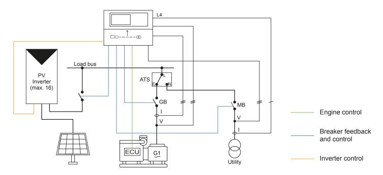
NOTE Alternatively, this application can have an externally controlled mains breaker.
