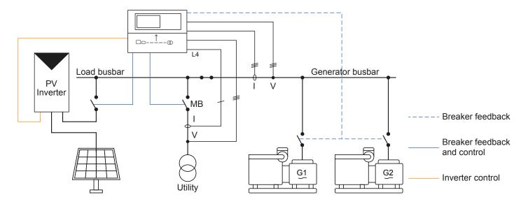
**NOTE** Alternatively, this application can have an externally controlled mains breaker.
