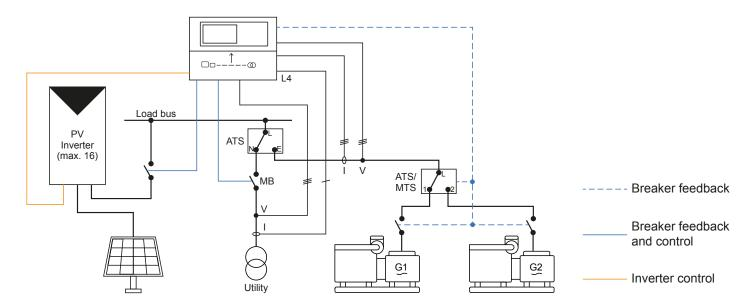
NOTE Use digital inputs and M-Logic for the feedback from the ATS and genset breakers.NOTE Alternatively, this application can have an externally controlled mains breaker.
