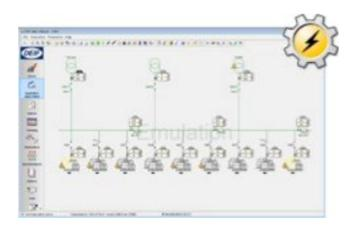
DEIF's Utility Software v.3 (USW-3) is a unique tool for engineers, service personel and end-users to configure and supervise one or several interconnected genset controllers, available for free download <u>here</u>.
