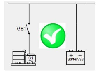
**Power source:** The battery is not intended to supply a load being the only source connected to the AC bus. Power source is used to take peak loads until genset start and improving power quality. The power reference is zero per default.
