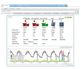
Example dashboard showing live values from a solar/diesel plant.
