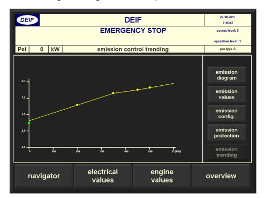
As an alternative, Lambda sensor emission control can be used. If Lambda is chosen in the gas mixer parameters, the mixer will be controlled based on the Lambda signal instead of the p/T signal.
