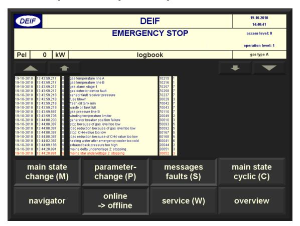
Offline mode: the triangular buttons are used to scroll up and down in the logs. The offline mode only shows the logs up to the time of selection of the offline mode. When scrolling, the view scrolls 18 indications, leaving the 19<sup>th</sup> from the previous view. If there are less than 19 logs, the upper line will be greyed out.
