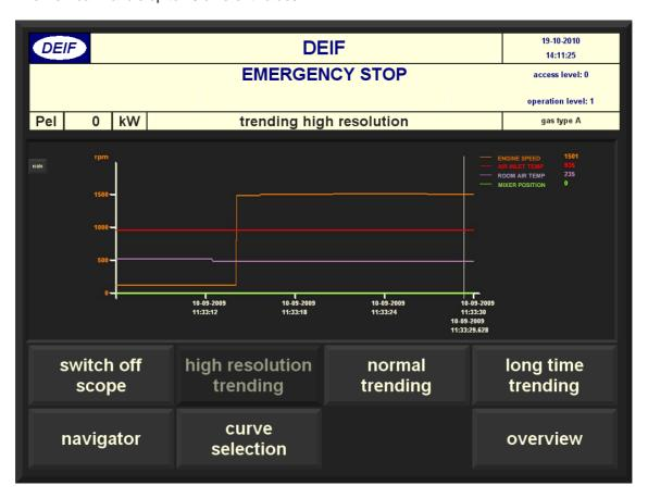
The small "scale" button in the top left corner by the side of the unit axis makes it possible to select the axis scaling to match the curves chosen.
